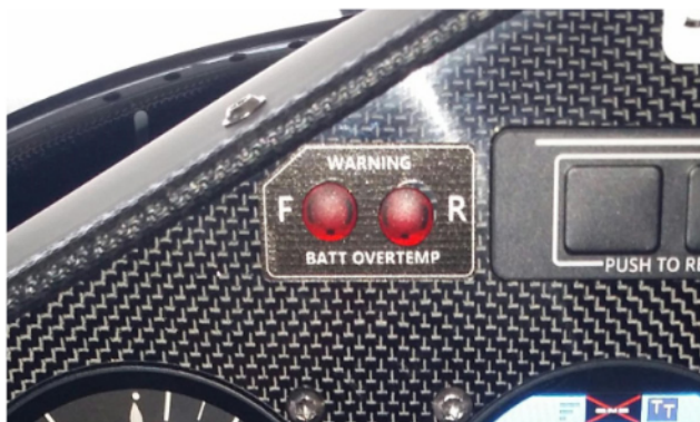
Battery overtemperature warning lights
