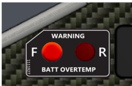
Example: front (F) battery overtemp warning light active
