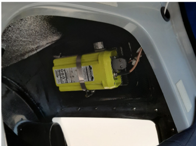
ELT transmitter location
